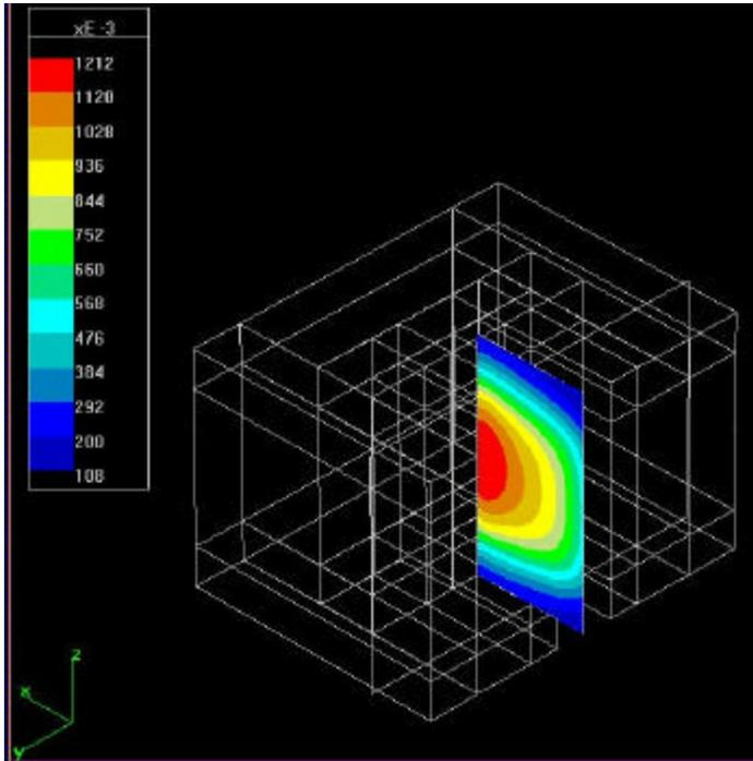
Figure 4: Field plot from a boundary element model, (Lorentz by IES).
