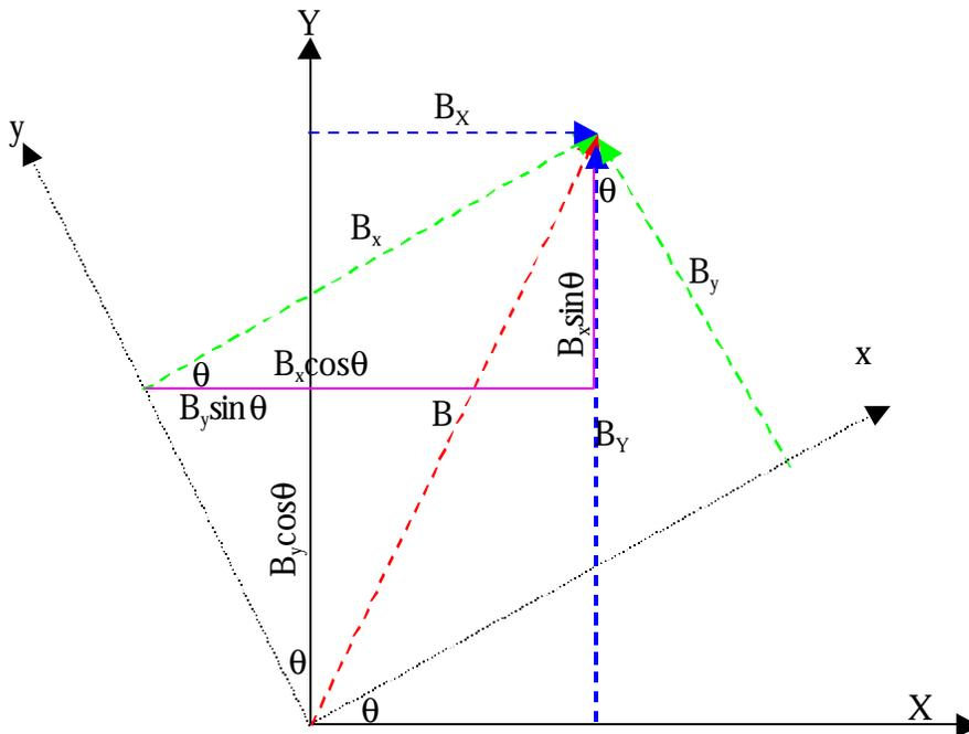
Figure 7: Construction diagram for the deduction of true magnet components.
