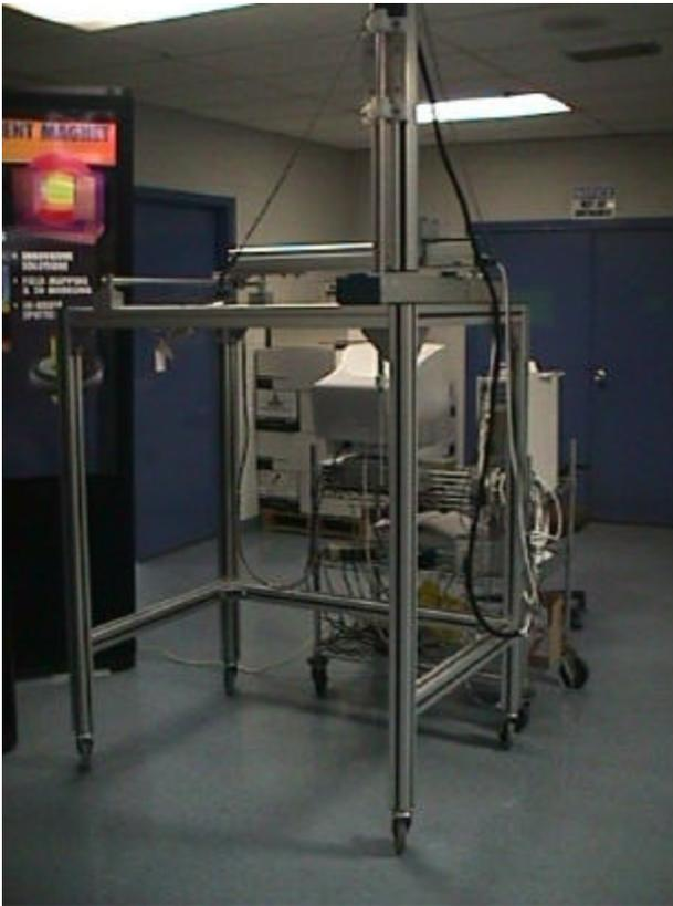
*Figure 2: Dexter Magnetic Technologies 3-Axis field Mapper.*
