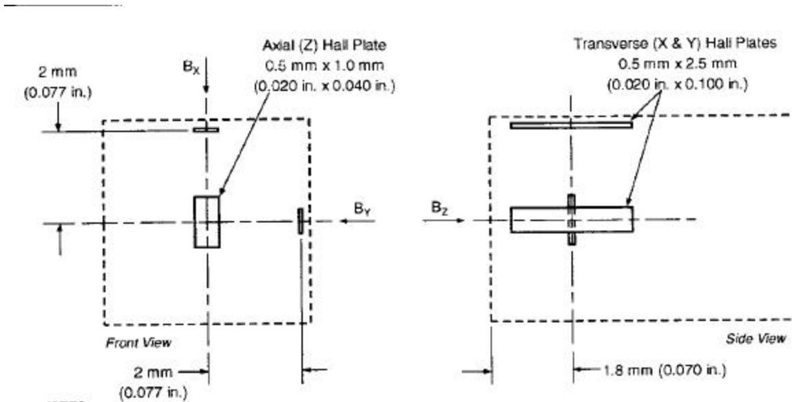
Figure 3: Example of layouts of hall elements within a 3-axis hall probe.
