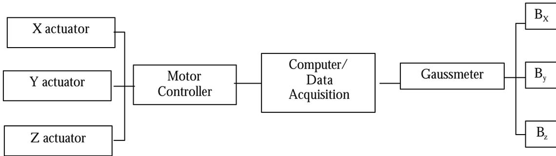
*Figure 1: Schematic of 3-Axis Magnetic Field Mapper*
