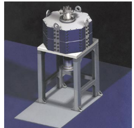
Figure 6 | 1 T Permanent Magnet and Vacuum Furnace Chamber
